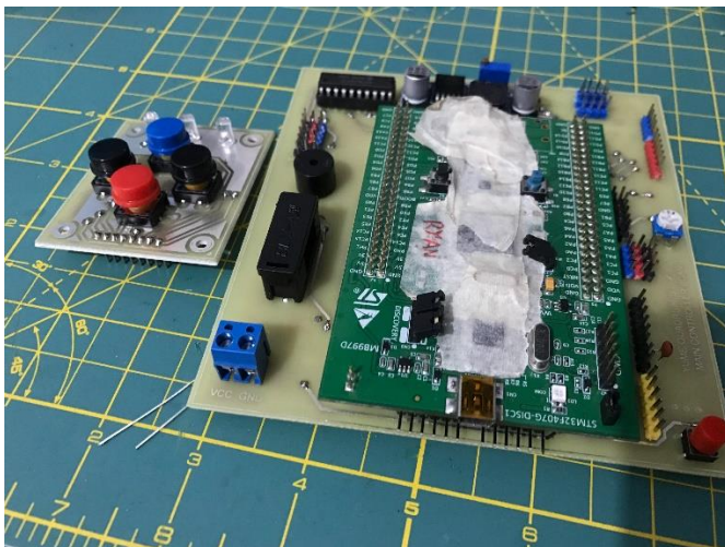
Gambar 3.16 Quadraped Robot Electronics Board
