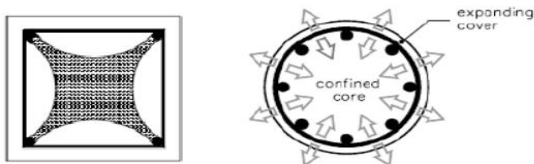
Gambar 2. 5. Efektifitas pengekangan. (a) sengkang persegi; (b) spiral
