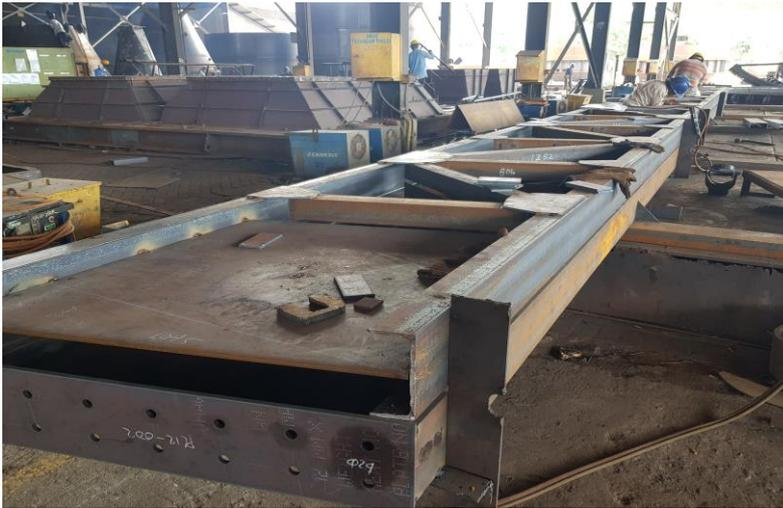
Gambar 4.6 Proses *fit-up* material
