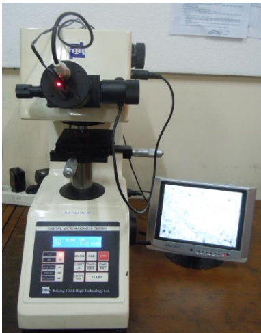
Gambar 3.5 Digital micro vickers hardness tester TH712
