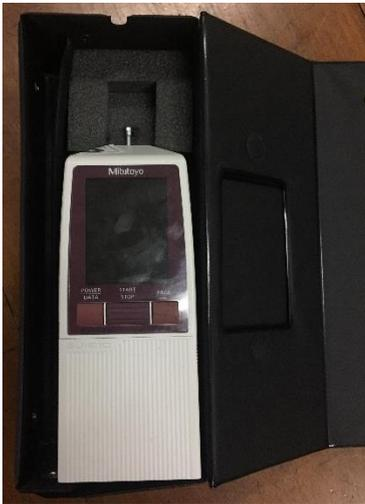
Gambar 3.3 *Surface Roughness Tester SJ-210*
