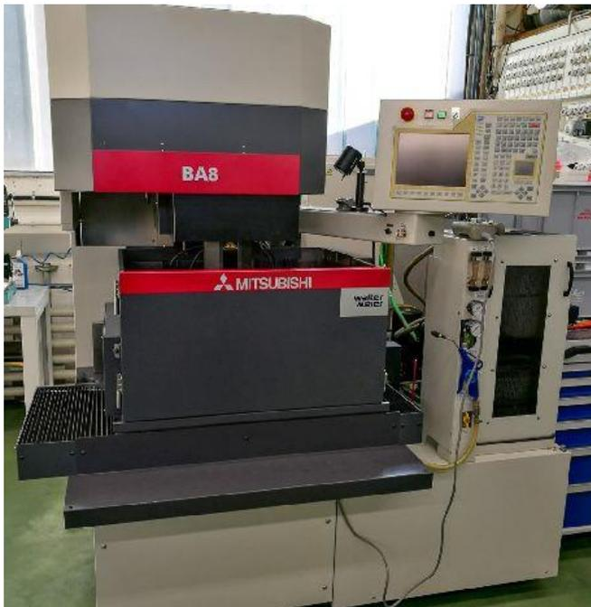
Gambar 3.2 Mesin *wire* EDM mitsubishi BA-8
