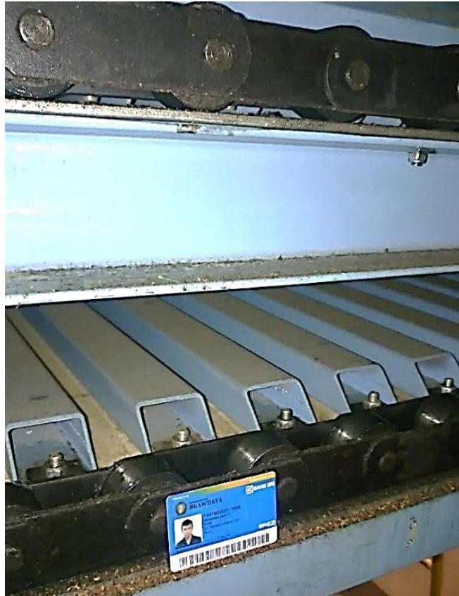
Gambar 2. 5 Roller Chain Conveyor
