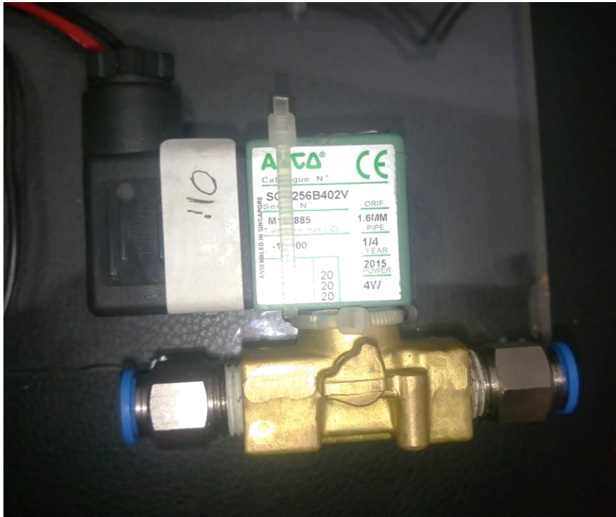
Gambar 2. 7 Solenoid Valve Tipe 2/2
