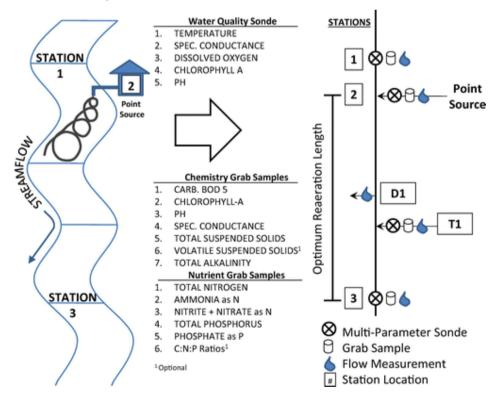
Gambar 2.1 Skema Qual2Kw
