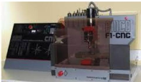
Gambar 2.8 CNC Milling TU-3A
