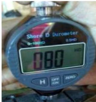
Gambar 2. 10 Shore D Durometer
