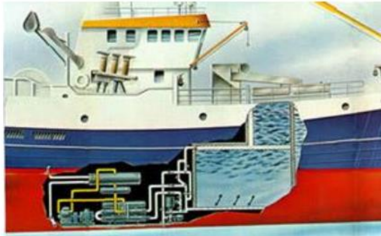
Gambar 4. Sistem Refrigerated Sea Water (Sumber: Effendi dan Indra, 2016)
