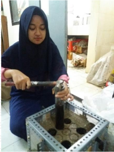
5. Instalasi Kolom Deep Soil Mixing (DSM)
