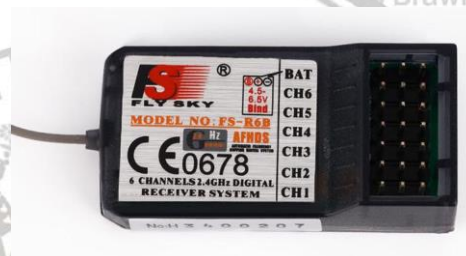
Gambar 2.7 Contoh receiver Fly Sky 6 kanal output
