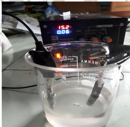
Gambar 4.13 proses *coating* plat besi ASTM A36 secara elektrofosis.
