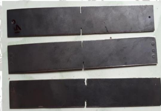
Gambar 4.9 Plat besi ASTM A36
