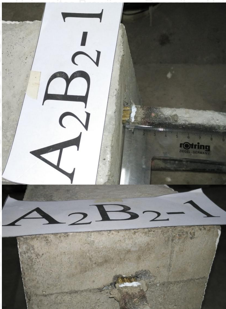
Gambar Keruntuhan Benda Uji Pull Out A 2 B 2 -1
