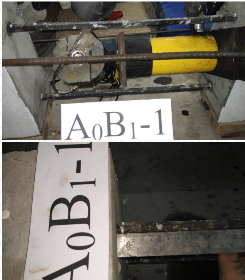
Gambar Keruntuhan Benda Uji Pull Out A 0 B 1 -1
