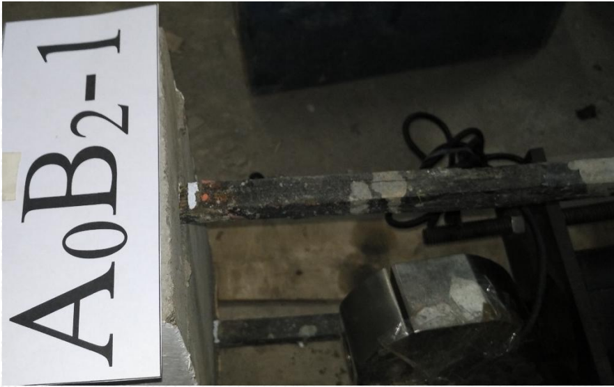
Gambar Keruntuhan Benda Uji Pull Out A 0 B 2 -1
