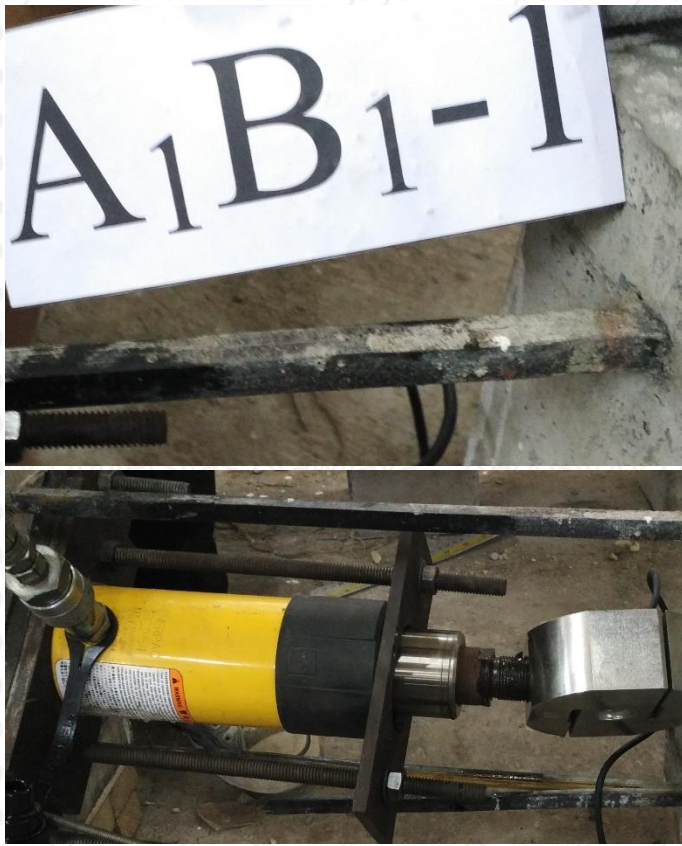
Gambar Keruntuhan Benda Uji Pull Out A 1 B 1 -1
