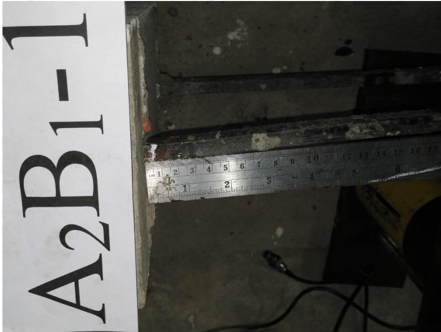
Gambar Keruntuhan Benda Uji Pull Out A 2 B 1 -1
