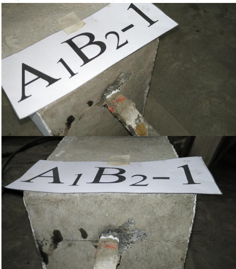
Gambar Keruntuhan Benda Uji Pull Out A 1 B 2 -1
