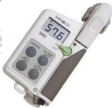
Gambar 5. Chlorophyll Meter Konika Minolta SPAD 502 (Sumber: http://www.makmursejati.co.id/wp-content/uploads/2013/04/Chlorophyll-Meter-SPAD-502-Plus.jpg )
