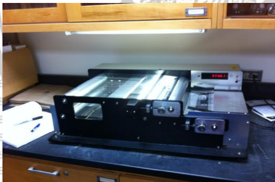
Gambar 4. Li-Cor LI 3100 Leaf Area Meter
