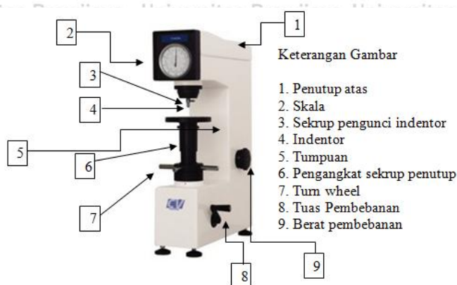
Gambar 3.2 Rockwell type hardness test
