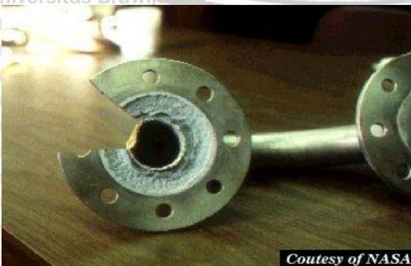
Gambar 2.16 *Crevice Corrosion*
