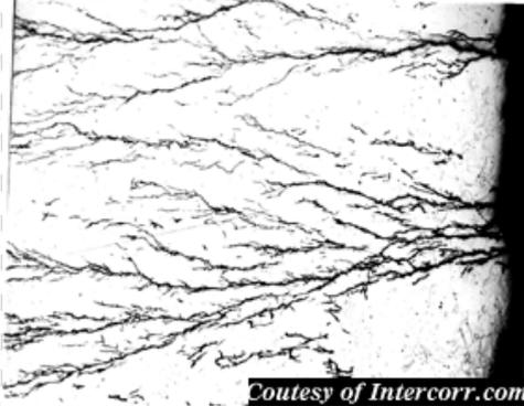
Gambar 2.15 *Stress corrosion*
