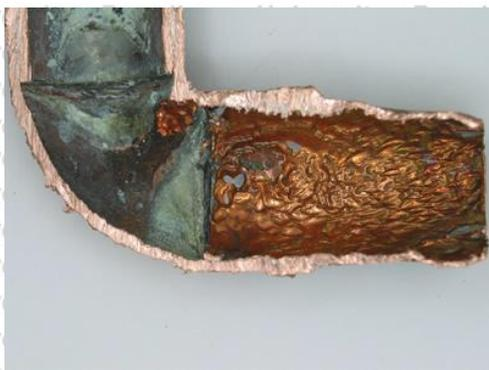
Gambar 2.12 Erosion corrosion
