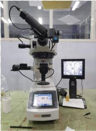
Gambar 3.4 Alat uji kekerasan *micro vickers hardness testing machines*
