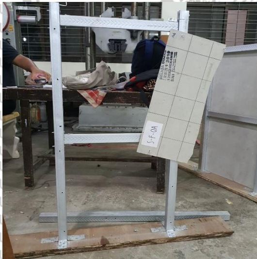
Gambar 4.25 Kondisi material fiber cement board saat mengalami sliding shear
