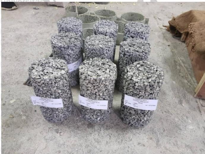
Gambar 4. 5 Benda uji beton porous
