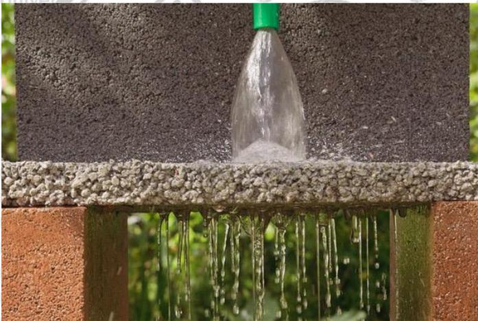
Gambar 2. 1 Beton porous
