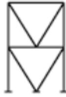
Gambar 2.12 V Bracing
