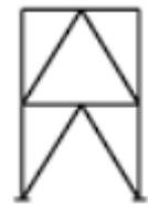
Gambar 2.13 Inverted V Bracing
