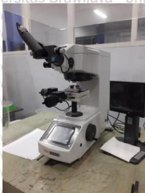
*Gambar 3.8 Micro vickers hardness testing machine*
