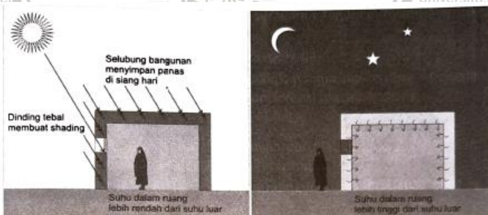
Gambar 2.2 Prinsip kinerja massa termal. Sumber: Idham, 2016
