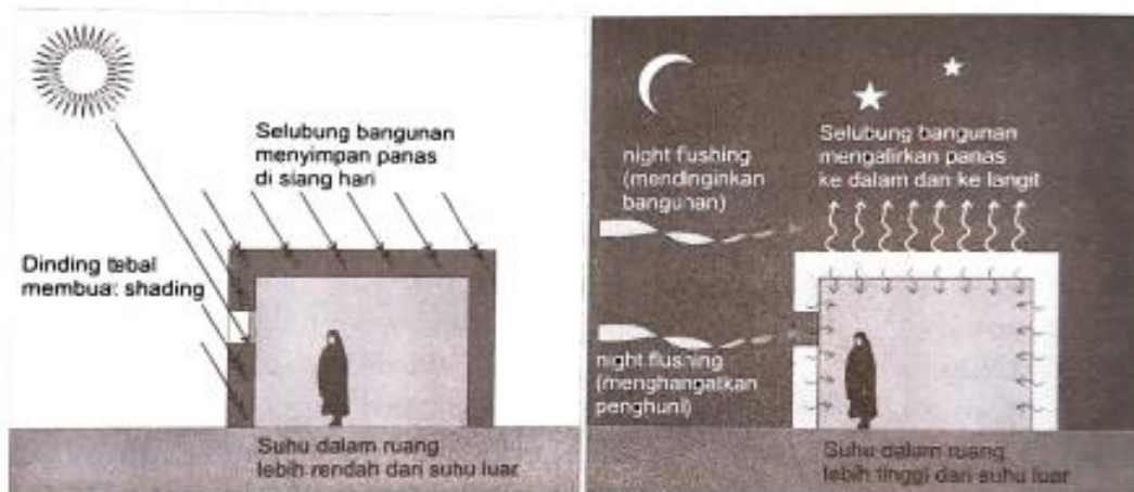
Gambar 2.6 Prinsip ventilasi night flushing . Sumber: Idham, 2016
