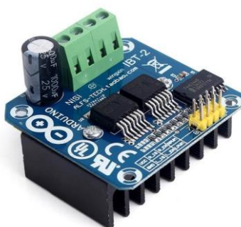
Gambar 2.10 Driver Motor H-Bridge BTS7960
