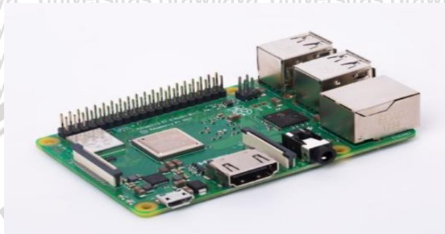
Gambar 4.4 Modul Raspberry Pi
