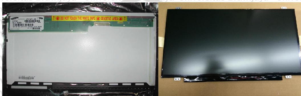
Gambar 4.6 Panel LCD 14 inch
