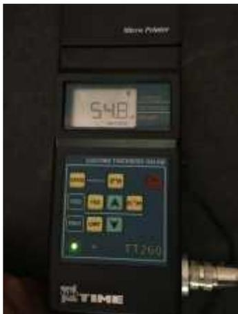
Gambar 3.11 Coating Thickness Gauge TT260
