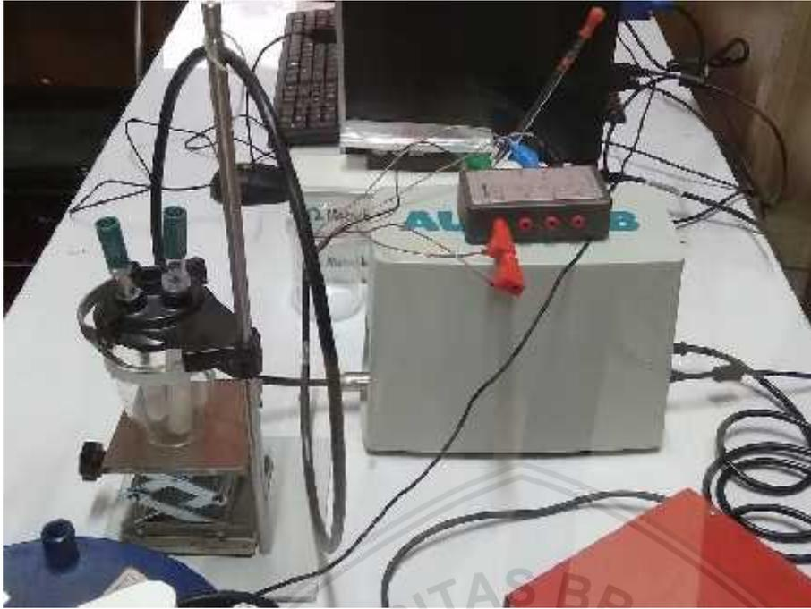
Gambar 3.10 Metrohm Autolab PGSTAT 204
