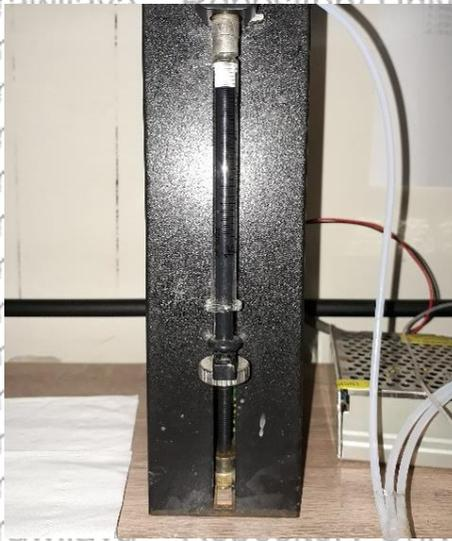
Gambar L.J.2 *Syringe pump SIA*
