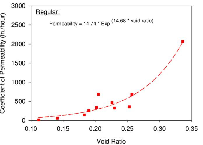
*Gambar 2.2 Relationship Between Pervious Concrete Void Ratio and Permeability*
