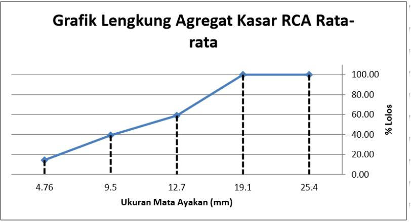
**Gambar 4.2 Gradiasi Agregat Kasar Daur Ulang (RCA)**
