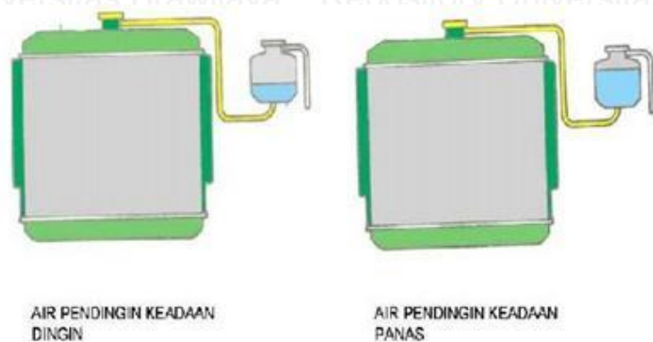
Gambar 2.7 Reservoir Tank Sumber: Irfan, S Ade. (2007)
