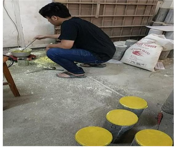
Gambar L 4.16 Proses *capping* benda uji silinder
