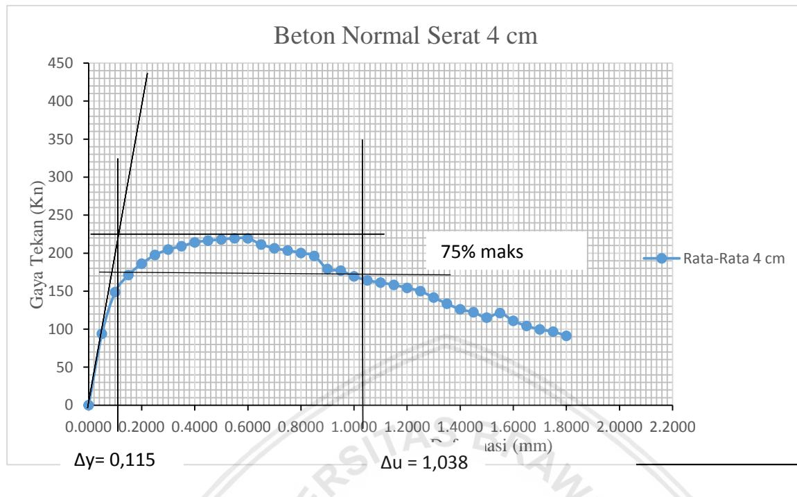
Gambar 4.17 Grafik proses perhitungan daktilitas initial tangen beton normal 4cm
