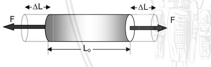
Gambar 2.6 Regangan (strain)
