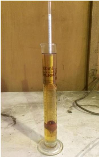
Gambar 3.9 Aerometer
