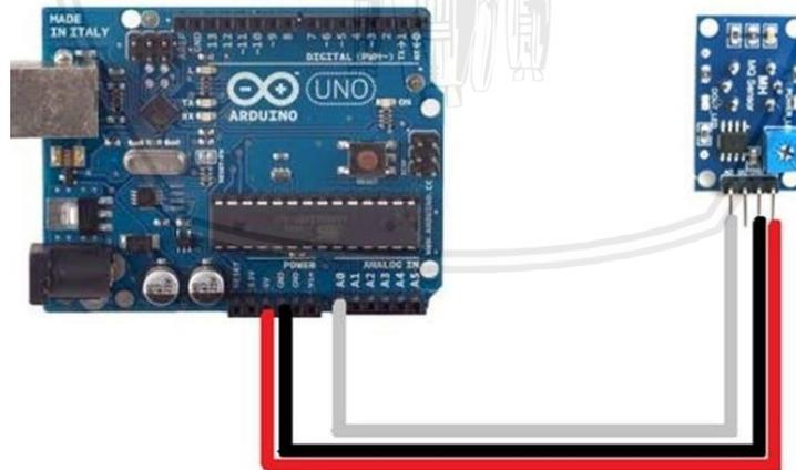
**Gambar 5.5 Skematik Sensor MQ135**
