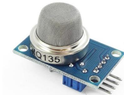
**Gambar 2.2 Sensor Gas MQ135**
