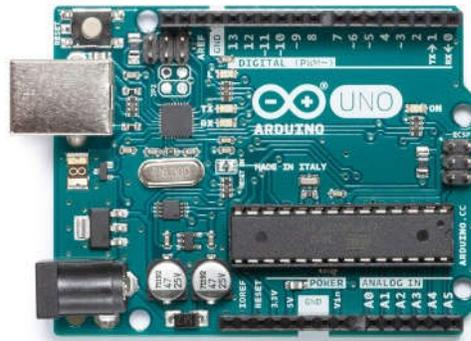
**Gambar 2.1 Mikrokontroler Arduino Uno R3**
