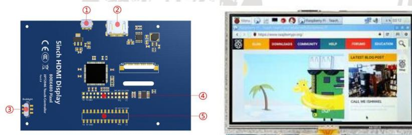
**Gambar 2.4 Fisik LCD (800x480) Touch Display for Raspberry Pi 2B**
