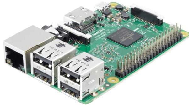
Gambar 2.3 Raspberry Pi 3 Model B
