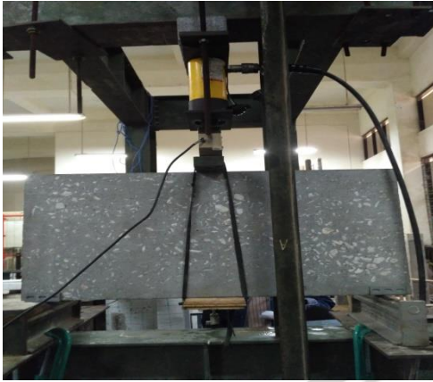
Gambar L 4.23 Pembebanan panel onyx
