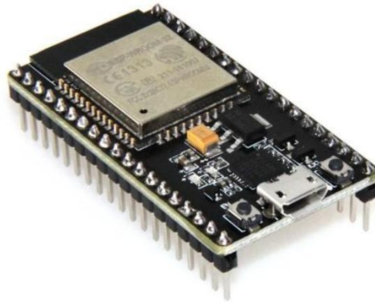
**Gambar 2.11** Papan ESP32 Dev Board
