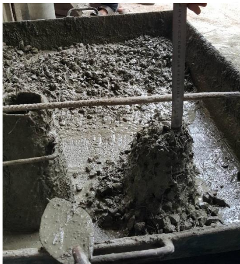
Gambar 4.2 Proses uji slump
