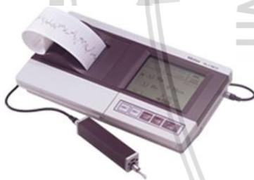
Gambar 3.2 *Surface Roughness Tester SJ-301*
