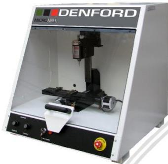
Gambar 2.5 Mesin *Micromill CNC Milling*
