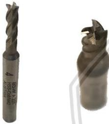
*Gambar 3.3 Square End Mill Diameter 4 mm*
