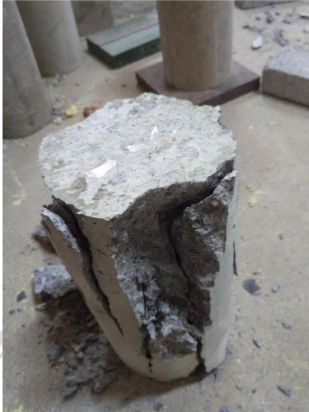
Beton RCA (*Recycled Coarse Aggregate*)
