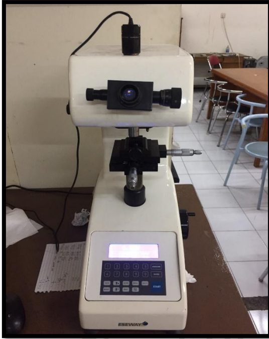
Gambar 3.5 Alat Uji Kekerasan Micro Vickers Eseway EW-412AAT
