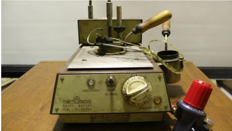
Gambar 3.3 Flash Point Tester
