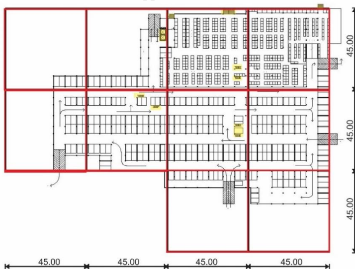
Gambar 4. 27 Emergency exit lantai basement tahap II
