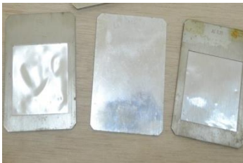
Filter Aluminium Pesawat Sinar-X
