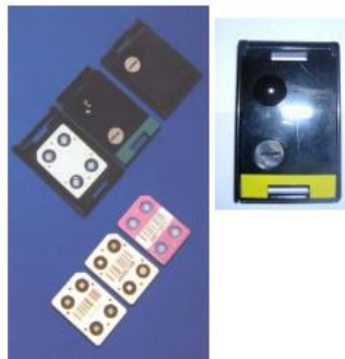
Gambar 2.5 Harshaw TLD card tipe 7776 dan holder tipe 8814 (Rofiq, 2006).
