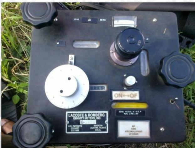
Gambar 3.3 Gravimeter LaCoste-Romberg Model G-1053
