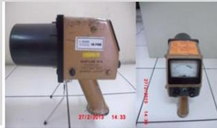
Gambar 2.10 Surveymeter model Babyline 61A
