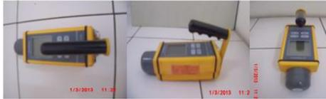
Gambar 3.3 Surveymeter (sinar-X)
