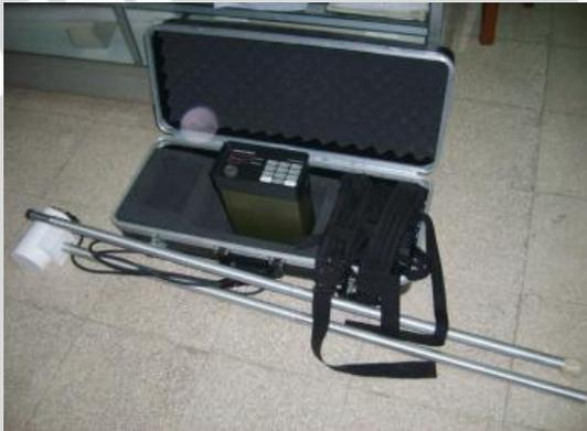
**Gambar 3.2** Proton Precision Magnetometer (PPM)
