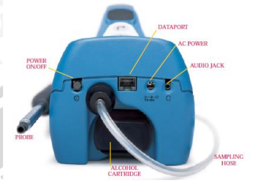
Gambar 2.1 Bagian-Bagian P-Track Particle Counter Model 8525
