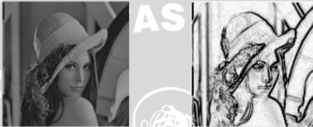
Gambar 2.13. Gambar Asli dan Hasil Sobel Edge Detection (Sumber: http://www.pages.drexel.edu )
