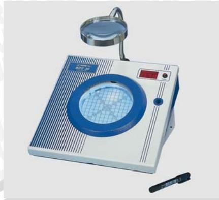
Gambar 4.1 Gambar Alat Colony Counter
